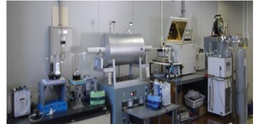
▲ Experimental apparatus for adsorption and reaction treatment of gaseous mercury
