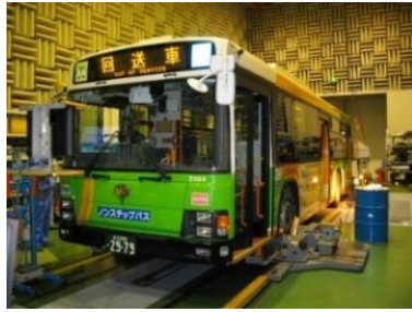
▲ Chassis dynamometer for large vehicles
