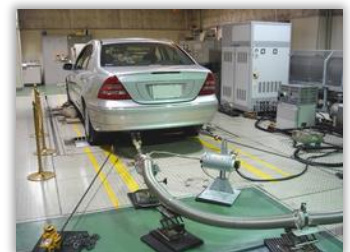
▲ Chassis dynamometer for a light-duty vehicle
