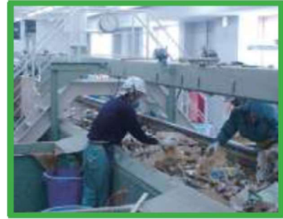
▲ Thorough pre-treatment is undertaken before automated treatment
