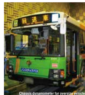
Chassis dynamometer for oversize vehicles
