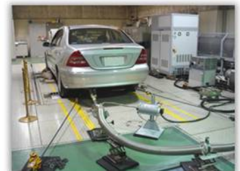
▲ Chassis dynamometer for a light-duty-vehicle
