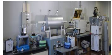
▲ Adsorption / reaction processing experiment apparatus in gaseous mercury
