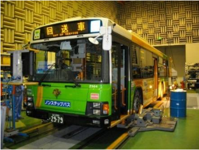
▲ Chassis dynamometer for heavy-duty-vehicles
